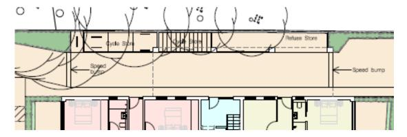
Image: Details of Refuse and Cycle Storage Area located along the northern boundary
